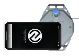
For **iPhones**: put the phone's top side against the edge of device where the QR code/NFC icon is located (dependent on model). The top frame of the phone should be touching or close to the base of the antenna. You will feel a vibration when the phone connects - do not move your phone.
