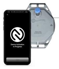
During the activation the app will show 'Device Activation in Process', ensure the back of your phone touches the device and is kept in the same position, for 10-30 seconds.
